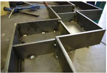
The staircase is open riser, clad with solid oak steps; the structure is fabricated in mild steel with a powder coated finish. The treads are made from folded steel trays, including associated glass clamps, fully clad with American White Oak so as to appear as if a solid piece.
